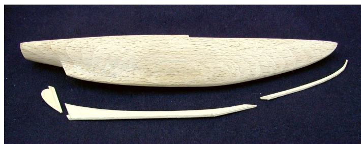
The kit hull and added keel and rudder. Note that the transom angle is incorrect - this was fixed after the picture was taken.
