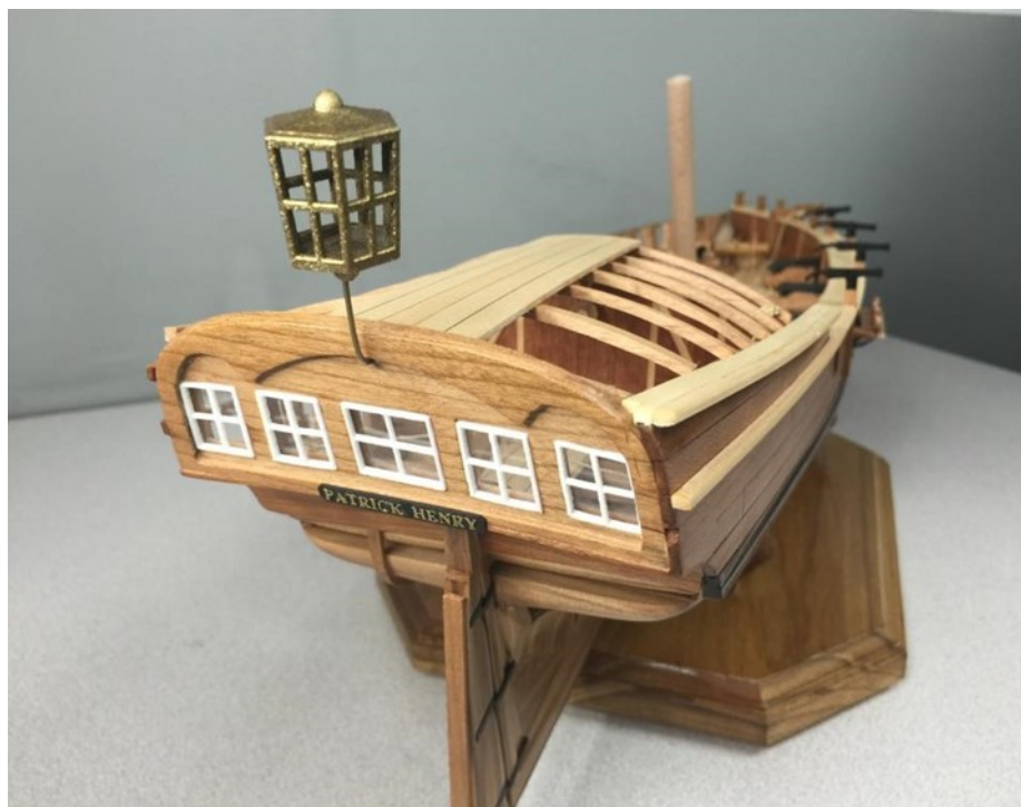
3D printed window frames and lantern was a kit first in 2015
